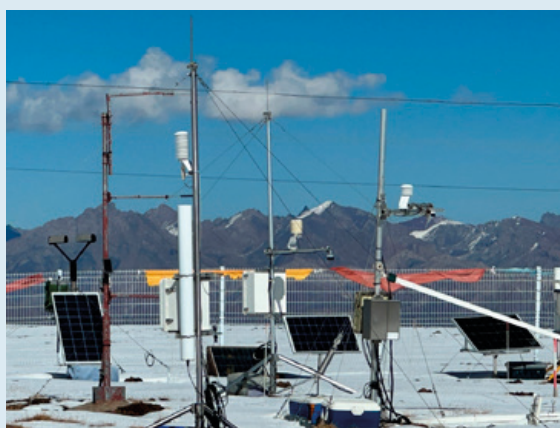
Example of an INARCH automated hydrometeorological station deployed to a high mountain basin: Qilian Mountains, China
